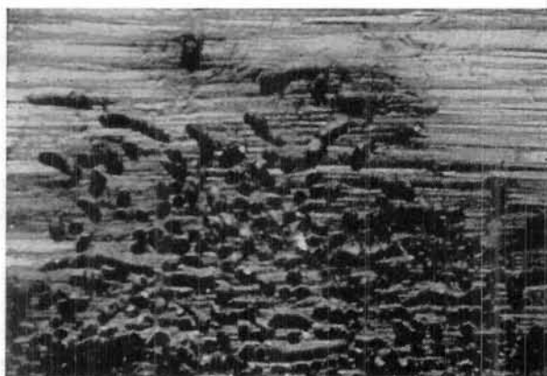
FIGURE 124.—Teredinidae: Douglas fir wood attacked by Teredo parksi .
