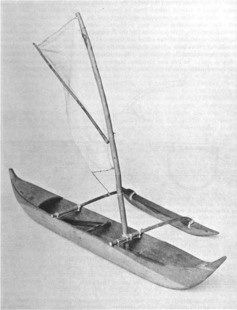
FIGURE 17.—Model of outrigger canoe from Bonin Islands (Science Museum, South Kensington, London): Hawaiian pseudo-frame replaced by cross brace of which ends perforate sides just under gunwale; European sprit sail; canoe body closely resembles that of Hawaii.
