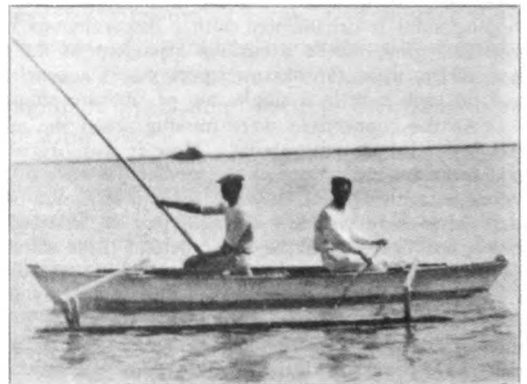
FIGURE 121.—Modern outrigger canoes of Manihiki, plank-built after a European model, with stem and stern posts to which side strakes are nailed; both ends covered in for a short distance; outrigger has two booms, each with a board attachment, consisting of two flat staves diverging upward from float to boom, which rests on their upper ends (from Buck, 1932).
