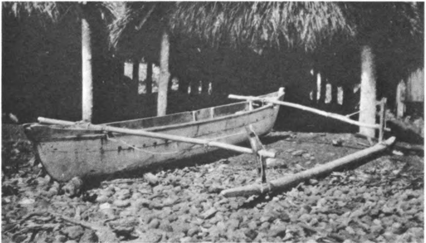
FIGURE 27.—Modern outrigger canoe ( vaka-poti ); differs from old type in being partially plank-built with short deck at each end and board connective replacing overcrossed stanchions (photographed in 1925 in Hivaoa, Marquesas).
