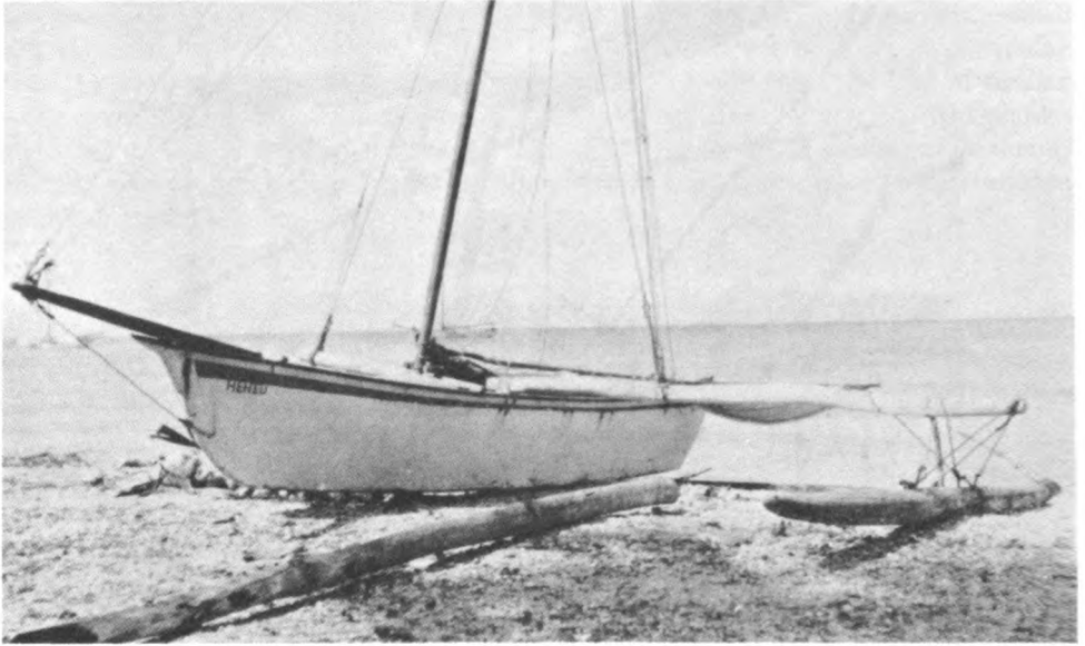
FIGURE 52.—Modern sailing outrigger of Fakarava; European rig has been adopted but outrigger is normal (photographed in 1925).
