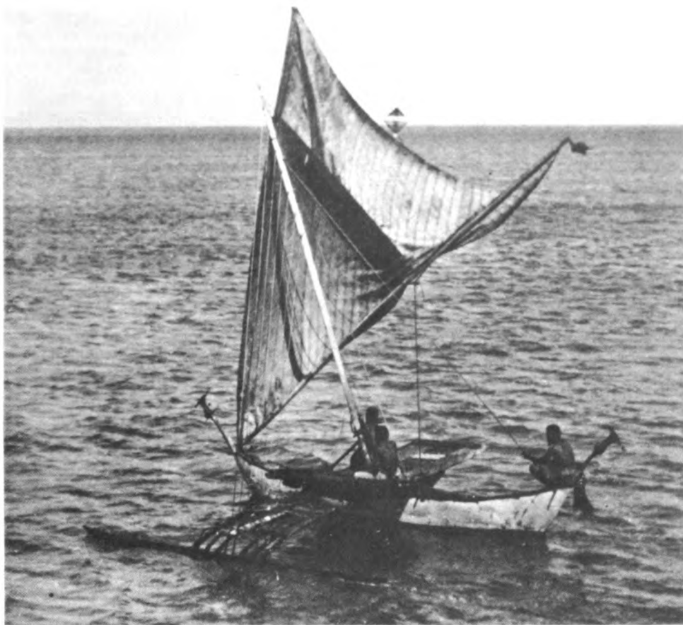
FIGURE 264.—Marshall Islands canoe under sail, photographed at Jaluit, 1900 (courtesy of U. S. National Museum). Shows method of reducing the sail area by the use of a spiller line—the line held by the steersman.
