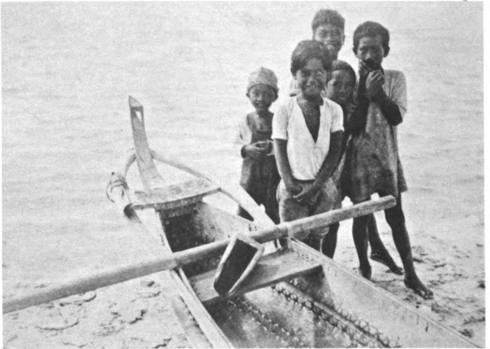
FIGURE 41.—Tatakoto fishing canoe of present day: a , stern curves up characteristically, booms project outboard to considerable distance on off side; b , details of stern showing steersman's seat stretching between two curved bars which represent head rails of Vahitahi type, bailer without handle rests on thwart (photographs by K. P. Emory).
