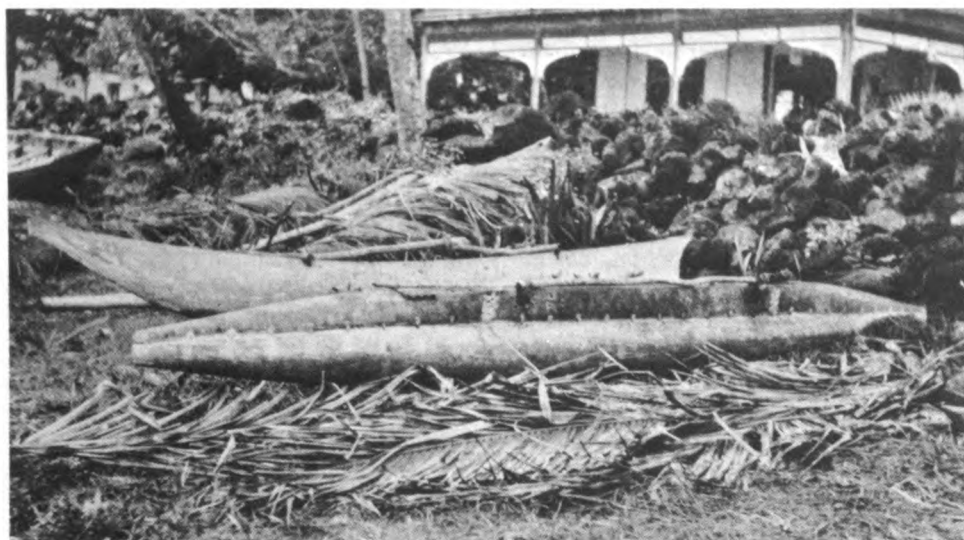
FIGURE 194.—Small fishing canoe of Niue: a , end view, head on, each end of hull covered by long whaleback end piece, rude gunwale rail present, batten covers washstrake seam inside, single stringer lies across booms, float cylindrical and bluntly pointed in front, truncate behind; b , side view showing torpedo shape of hull, short median washstrake, and long end pieces, Samoan paopao in background (photographed at Apia, 1925).
