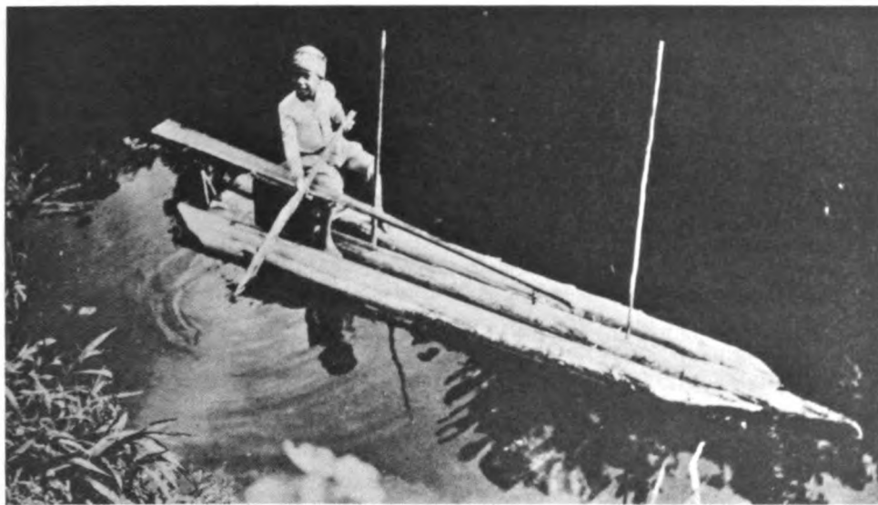
FIGURE 32.—Catamaran made of three banana stalks skewered together (photographed in 1925 in Taipi Valley, Nukuhiva).
