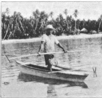
FIGURE 121.—Modern outrigger canoes of Manihiki, plank-built after a European model, with stem and stern posts to which side strakes are nailed; both ends covered in for a short distance; outrigger has two booms, each with a board attachment, consisting of two flat staves diverging upward from float to boom, which rests on their upper ends (from Buck, 1932).
