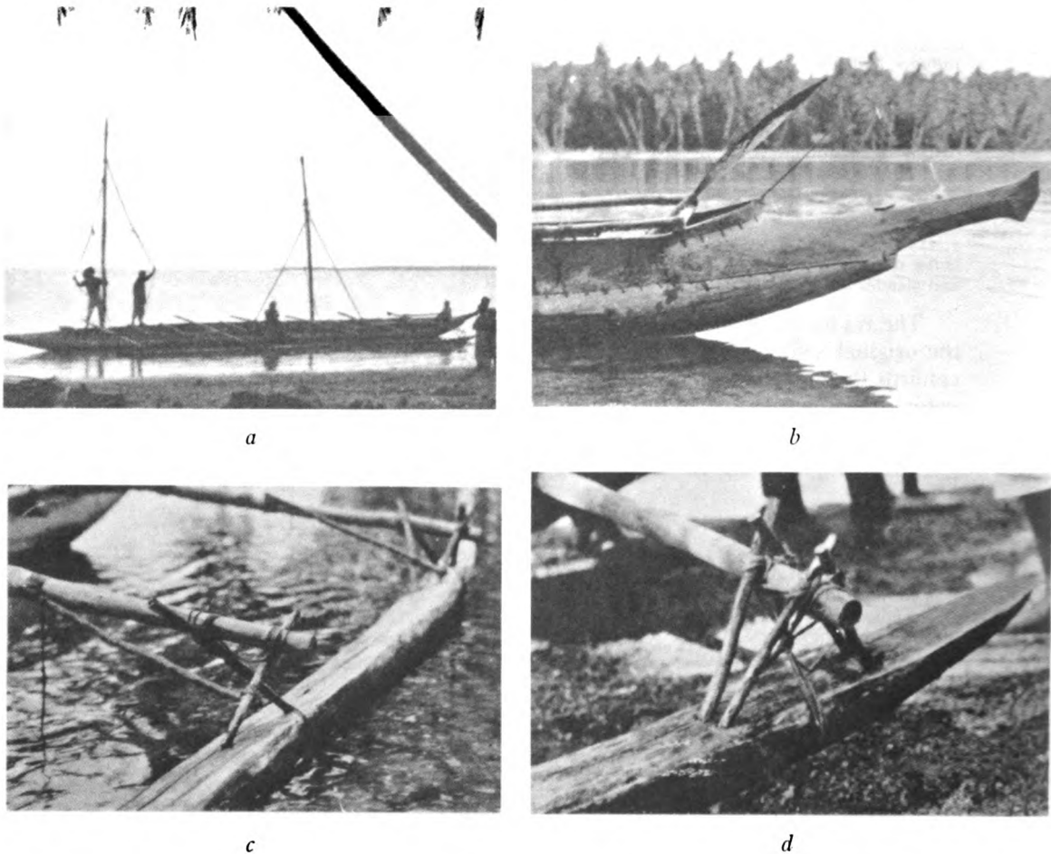
FIGURE 179.—Pukapuka canoes. a , large two-masted outrigger canoe, only one surviving: length 60 feet; six booms connect indirectly with float and six false booms connect with a long stringer placed fore and aft over true booms about half-way outboard; each mast has a fore and an after stay; prow is horizontal and obtusely pointed; stern slightly sheered, ending in truncate knob. b , stern of same canoe showing details; single diamond-shaped carving in low relief on stern piece probably represents vestigial knob to which egg-cowries are attached in Samoan and other outriggers in a similar position. c , two forms of outrigger attachment, same canoe: farther attachment consists of two pairs of converging overcrossed stanchions of ordinary Tokelau type, strengthened by an oblique accessory rod attached at inner end to boom and at outer end to one of the inner pair of stanchions, and by an X-shaped suspensory lashing which makes several figure-of-eight turns around boom below and lashed-on ends of stanchions above, finished off by several turns at point of crossing midway between boom and float; this type characterizes attachment of outermost boom at each end of the set of six; attachments of the inner four, of which one is seen in foreground, are reduced to a single pair of undercrossed stanchions; an oblique accessory rod and a wire suspensory lashing are present. d , aftermost outrigger attachment of small canoes, similar to the form typical of the canoes of the western Tokelau Islands, no oblique accessory rod being present. In this and in all other Pukapuka canoes the float is flat above, rounded below; it is a straight log, the fore end horizontal, the after one slightly sheered to a flat-topped point. (Photographs by the Templeton Crocker Expedition, 1933.)
