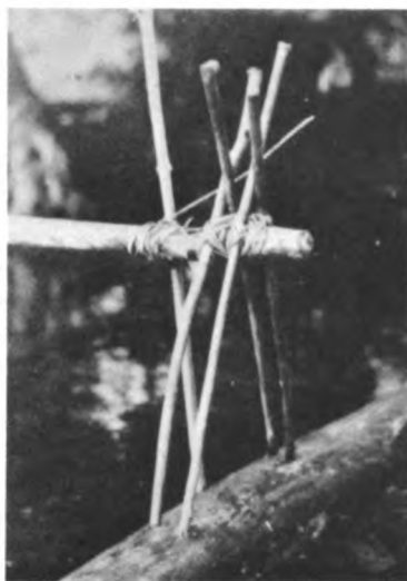
FIGURE 41.—Connectives of a lake canoe, Rennell Island (Templeton Crocker Expedition, 1933).
