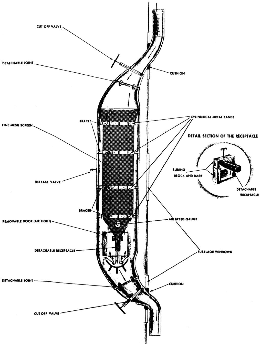
Fig. 1. Preliminary diagram of internal airplane trap. The actual trap produced varies in several aspects.
