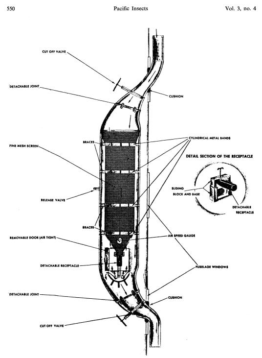
Fig. 1. Preliminary diagram of internal airplane trap. The actual trap produced varies in several aspects.
