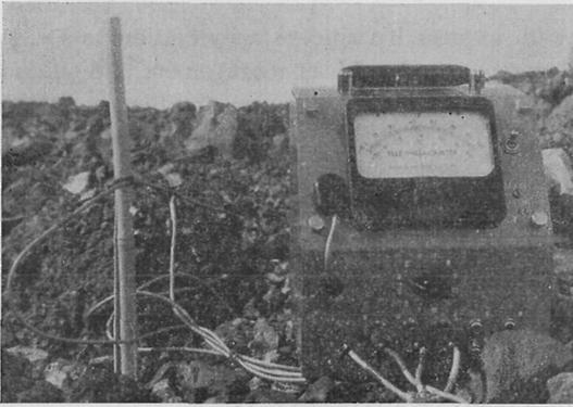
Fig. 1. Portable instrument used for recording soil and air temperature.
