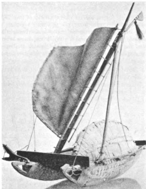
FIGURE 37.—Two-masted double voyaging canoe with Oceanic lateen sail, Fagatau, Tuamotu Archipelago, model made by native "about 1854" (B. P. Bishop Mus., no. 3474).
