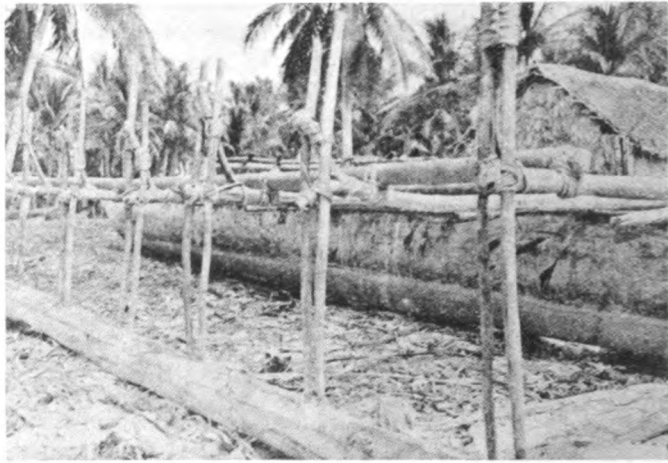
FIGURE 3.—Forked booms with parallel stick or clamp connectives, Tupuselei, Keapara area, Central Division, Papua (photograph by Kathleen Haddon).
